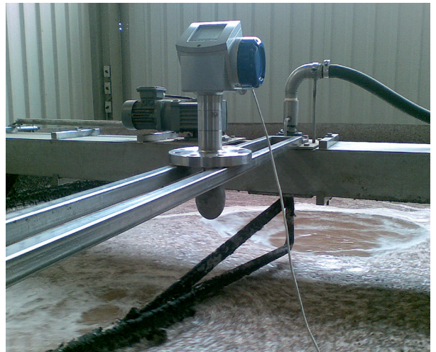
When foam builds up under the measuring device, the foam removal mechanism is activated
