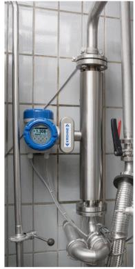
Brix measurement with the OPTIMASS 7300
