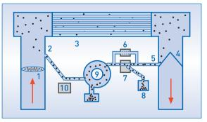
Process scheme of a condenser tube cleaning system
