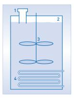
Each tank has the shape of an upright barrel with a diameter of about 3.5 m and a total height of approx.15 m. It has heating coils at the bottom and an agitator in the center. There is a 150 mm thick insulation all over the tank top which includes a nozzle ( $\emptyset$  150 mm / 250 mm high). The measuring device is to be installed on the nozzle and give accurate and reliable measuring values despite condensation from the hot product, its high viscosity and low dielectric constant.
