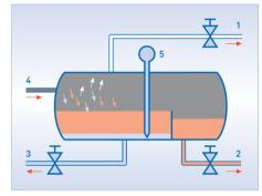
1 Gas, 2 Oil, 3 Water, 4 Crude (Oil/Gas/Water/ Sediments), 5 OPTIFLEX 1300 C
