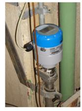
OPTIFLEX 1100 with reduced process connection
