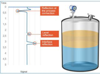
Schematic drawing on interface measurement with TDR technology
