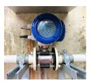
Flow measurement of aluminium sulphate with the OPTIFLUX 7300 C
