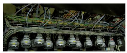
Measurement of the metered flavours using OPTIFLUX 6000 and OPTIMASS 3000.
