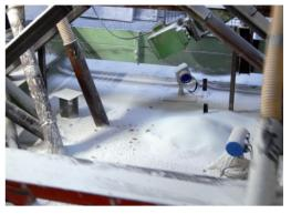
Level measurement of glass granulate using the OPTIFLEX 1300
