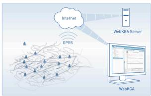
Schematic layout of measuring points with GPRS module
