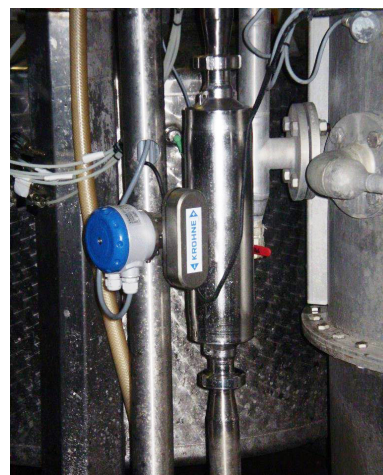
Fermented potato mash measurement with the OPTIMASS 1300
