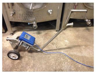
Portable measuring device incorporating the OPTIFLUX 2100
