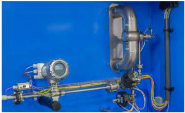
Process instrumentation for the CIP (Clean in Place) system: Stock management with the OPTIFLEX 2200 level transmitter (top and centre left). Dosing of CIP agents (bottom) and flow measurement of the CIP lines (top/centre right).
