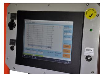
Recording unit of the grout monitoring system
