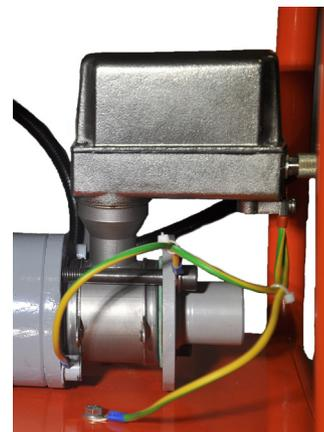
BATCHFLUX 5500 on mobile grout monitoring system
