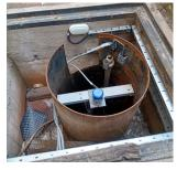
Measurement of water level in a lock chamber
