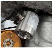
Hydrostatic level measurement of vegetable oil with the OPTIBAR PM 3050
