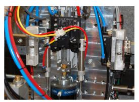
Variable area flow measurement of coolant
