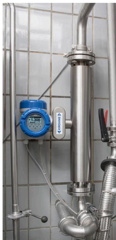
Brix measurement with the OPTIMASS 7300
