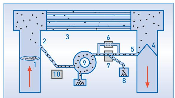
Process scheme of a condenser tube cleaning system
