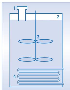
Each tank has the shape of an upright barrel with a diameter of about 3.5 m and a total height of approx. 15 m. It has heating coils at the bottom and an agitator in the center. There is a 150 mm thick insulation all over the tank top which includes a nozzle (Ø 150 mm / 250 mm high). The measuring device is to be installed on the nozzle and give accurate and reliable measuring values despite condensation from the hot product, its high viscosity and low dielectric constant.
