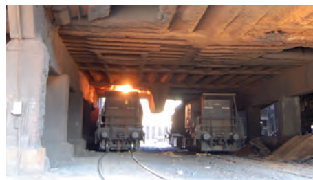
Filling a torpedo ladle car
