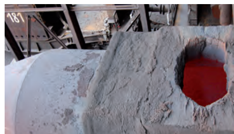
Steel ingress hole on top of a car
