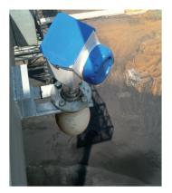
OPTIWAVE 6300 C fitted on conveyor
