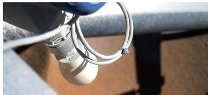
OPTIWAVE 6300 C with DN 80 (3") PP Drop antenna on tripper conveyor measuring level of stock pile
