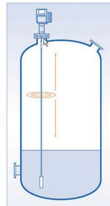
Mesuring principle of the Guided Radar (TDR) level meter OPTIFLEX 1100
