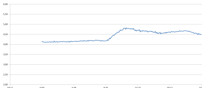
Change in sludge level of flocculation tank when polymer is omitted (simulation)
