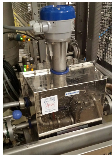
Dosing liquid chocolate using the OPTIMASS 6400 (with heating jacket)
