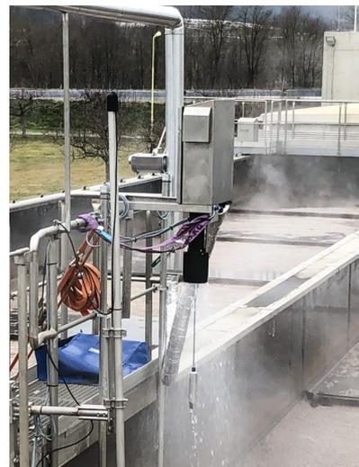
Integrated flush cleaning for the sensor
