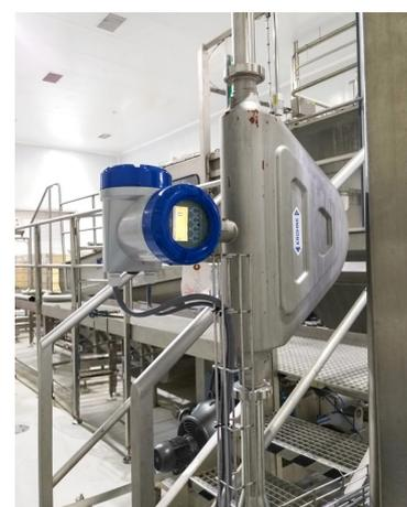
Flow measurement of tomato paste with the OPTIMASS 6400 C
