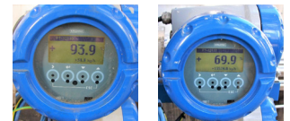
Sulphuric acid concentration measurement (left: undiluted, right: diluted)
