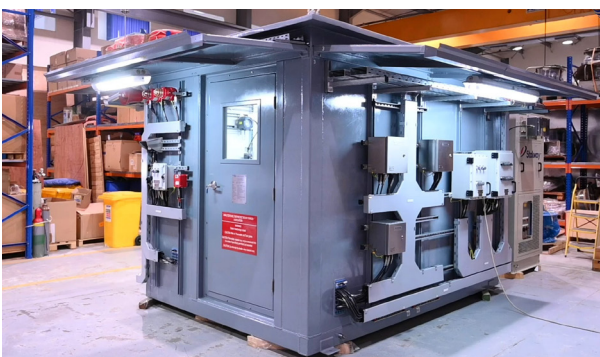
Analyzer house and shelter with gas analyzers for sour gas analysis
