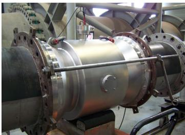
OPTIFLUX 4300 on calibration rig
