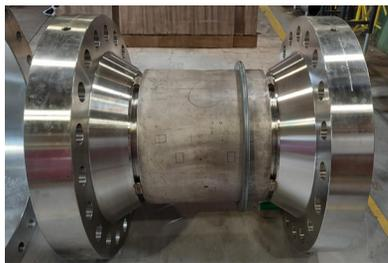
Production of KROHNE 24" flow sensor with high pressure flanges
