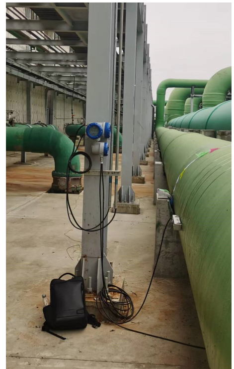
Non-invasive flow measurement of saltwater with the OPTISONIC 6300
