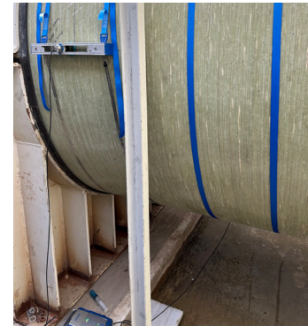
Battery-powered ultrasonic clamp-on flowmeter with portable signal converter
