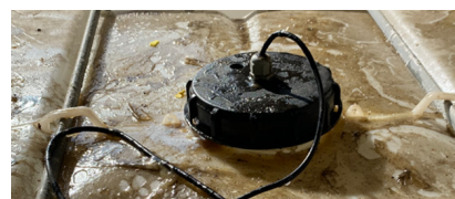
Pressure level sensor previously installed in the IBC tanks
