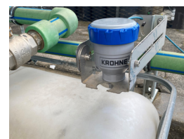
Level measurement through the IBC plastic roof top
