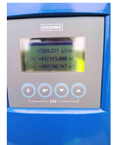
Conductivity and totalised volume flow of manure displayed on the flow converter of a KROHNE EMF
