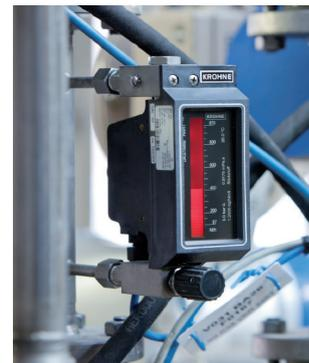
Nitrogen flow measurement with the DK 37
