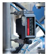
Nitrogen flow measurement with the DK 37
