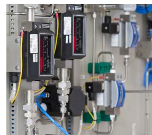
Reference gas and inert gas measurement with DK37 and DK34
