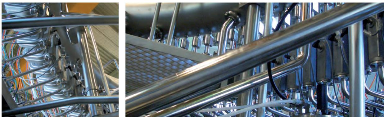
OPTIBATCH 4011 C on the filling machine (seen from the inside)
