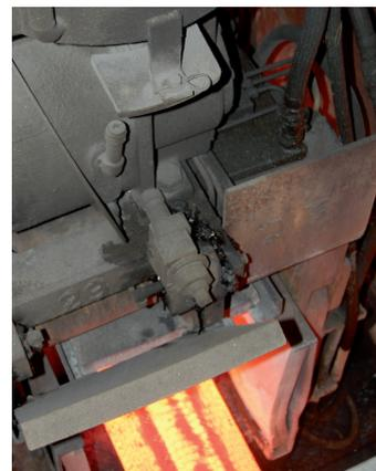
Measuring insert of a Pt100 sensor in the gear mechanism of the drive motor
