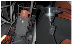
OPTITEMP TRA-P14 connection head mounted on water-cooled motor cladding
