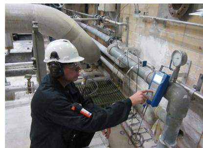
The OPTISONIC 6300 P with mobile signal converter attached to a pipeline
