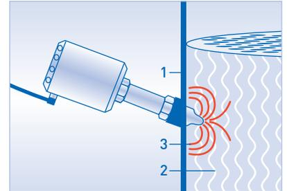
1 Wall of mash filter, 2 Medium, 3 Line of electric flux
