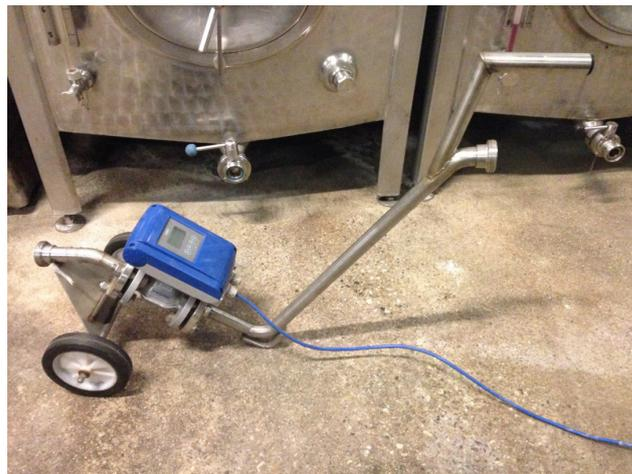
Portable measuring device incorporating the OPTIFLUX 2100
