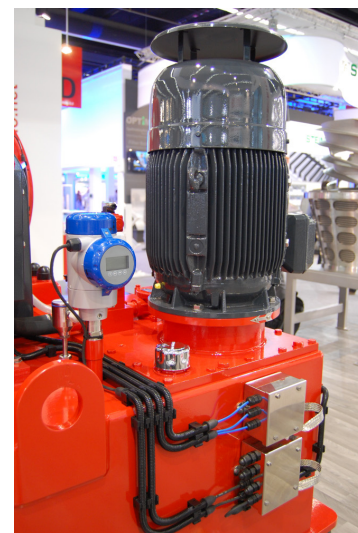
Oil level monitoring in a pusher centrifuge with the OPTIFLEX 2200 C
