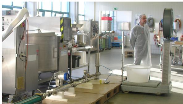
Test installation with the OPTIMASS 7400 C
