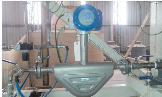
Unaffected by vibrating environment: OPTIMASS 6400 C
