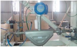
Unaffected by vibrating environment: OPTIMASS 6400 C
